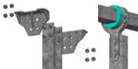
Fig. 2. Washer Joints are Used for the Assembly of these structures very Often.
