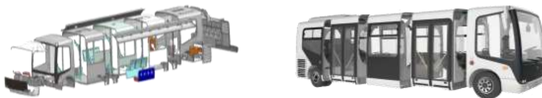
Fig. 1 Modular composite structure and monocoque bus design.
