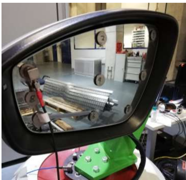
Fig. 1 Measurement of operating waveforms of rearview mirror oscillations
